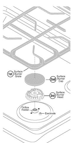
To Remove and Replace the Surface Burner Caps and Burner Heads - Remove in the following order: (1st) surface Burner Grates, (2nd) Burner Caps and (3rd) Burner Heads. Reverse the procedure above to replace the surface Burner Caps, Burner Heads and Burner Grates.
